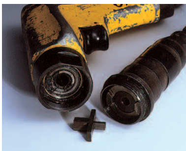
Damaged pneumatic tooling
